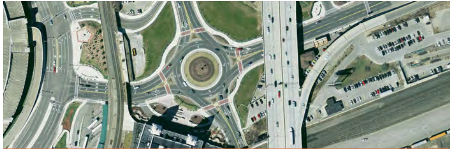
WORCESTER, WASHINGTON SQUARE URBAN MULTILANE ROUNDABOUT
